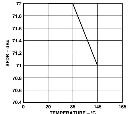
Figure 13. SFDR vs. Temperature @  $f_{CLOCK} = 50$  MHz, ( $f_{OUT} = 1$  MHz)
