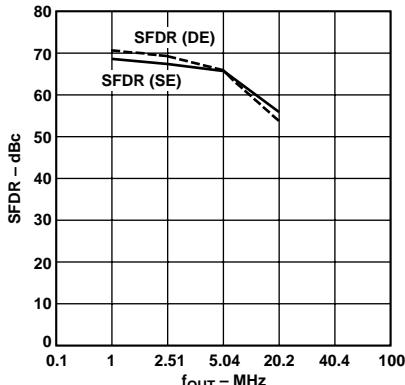
Figure 12. SFDR vs.  $f_{OUT}$  @  $f_{CLOCK} = 140$  MHz (Single Ended and Differential)
