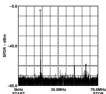
Figure 18. Single-Tone SFDR @  $f_{CLOCK} = 140$  MHz ( $f_{OUT1} = 20$  MHz)
