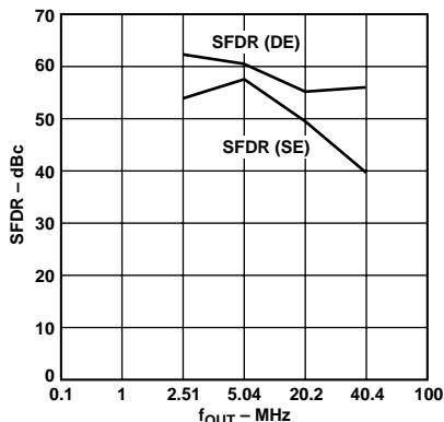
Figure 2. SFDR vs.  $f_{OUT}$  @  $f_{CLOCK} = 140$  MHz (Single Ended and Differential)
