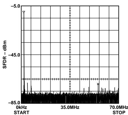
Figure 17. Single-Tone SFDR @  $f_{CLOCK} = 140$  MHz ( $f_{OUT1} = 2$  MHz)
