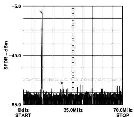
Figure 19. Dual-Tone SFDR @  $f_{CLOCK} = 140$  MHz ( $f_{OUT1} = 13.5$  MHz,  $f_{OUT2} = 14.5$  MHz)
