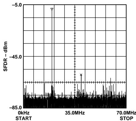
Figure 9. Single-Tone SFDR @  $f_{CLOCK} = 140$  MHz ( $f_{OUT1} = 20$  MHz)
