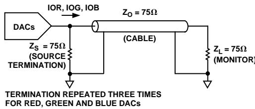
Figure 22a. Analog Output Termination for RS-343A
