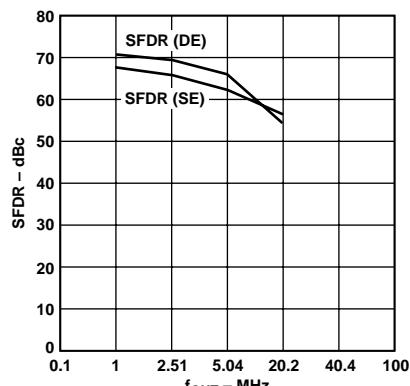
Figure 3. SFDR vs.  $f_{OUT}$  @  $f_{CLOCK} = 50$  MHz (Single Ended and Differential)
