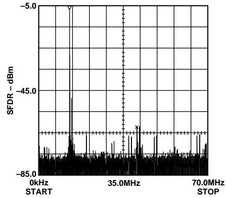
Figure 10. Dual-Tone SFDR @  $f_{CLOCK} = 140$  MHz ( $f_{OUT1} = 13.5$  MHz,  $f_{OUT2} = 14.5$  MHz)
