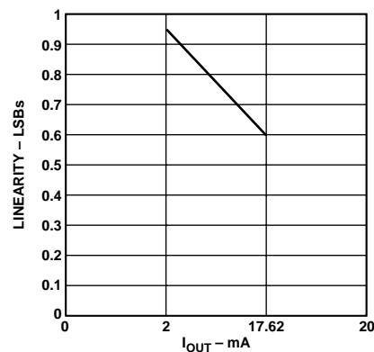
Figure 6. Linearity vs.  $I_{OUT}$
