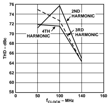
Figure 5. THD vs.  $f_{CLOCK}$  @  $f_{OUT} = 2$  MHz (2nd, 3rd and 4th Harmonics)
