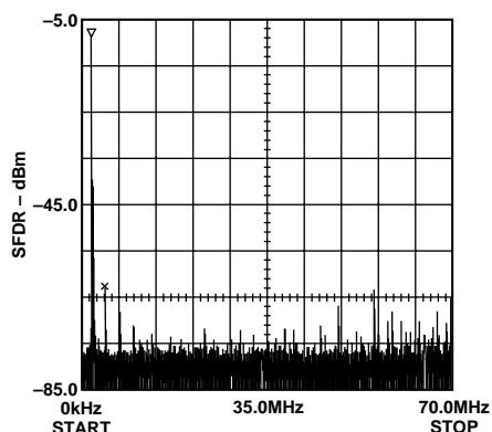
Figure 8. Single-Tone SFDR @  $f_{CLOCK} = 140$  MHz ( $f_{OUT1} = 2$  MHz)
