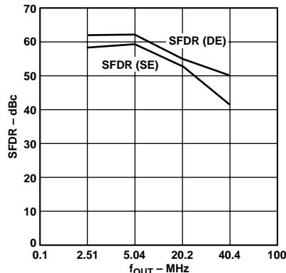
Figure 11. SFDR vs.  $f_{OUT}$  @  $f_{CLOCK} = 140$  MHz (Single Ended and Differential)
