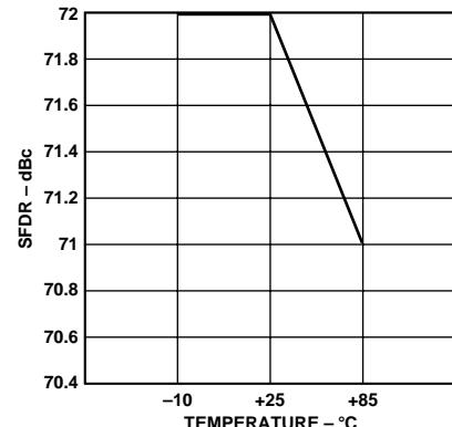
Figure 4. SFDR vs. Temperature @  $f_{CLOCK} = 50$  MHz ( $f_{OUT} = 1$  MHz)
