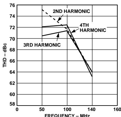
Figure 14. THD vs.  $f_{CLOCK}$  @  $f_{OUT} = 2$  MHz (2nd, 3rd and 4th Harmonics)
